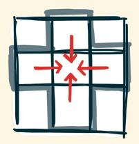
**Stencil computations** are a class of kernels which update *neighboring* array elements according to a fixed pattern, called *stencil*.
